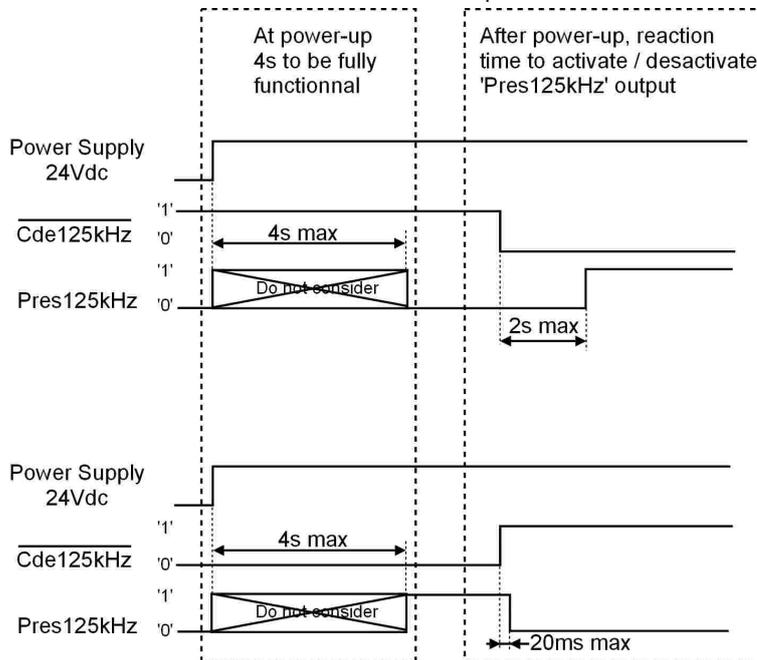
**Receiver test behavior via Data Rx**
