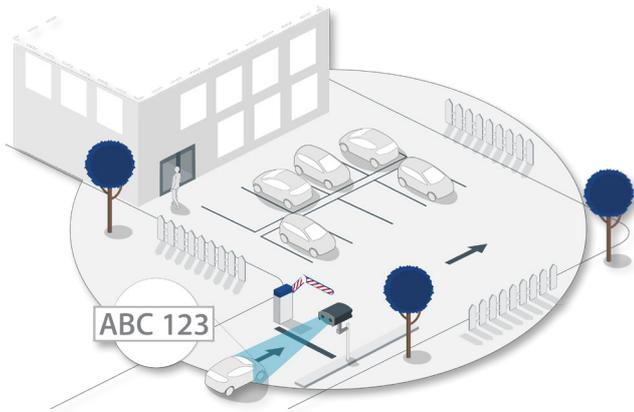
ANPR cameras have built in relays to provide automatic access control directly from the camera to open gates or barriers on a database match.
